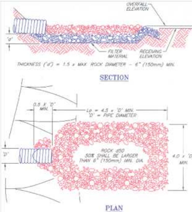
**TYPICAL ENERGY DISSIPATOR**
