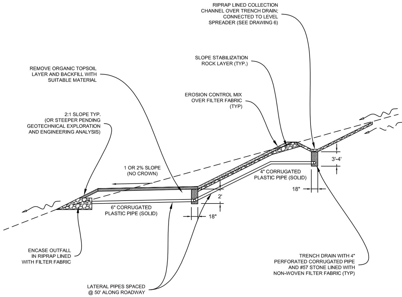
Note: The above drawing represents a situation where the roadway cuts into an existing slope with shallow groundwater; which is managed using the drainage blanket or trench drains. These measures would not be necessary if the roadway does not cut into the subsurface drainage layer.
